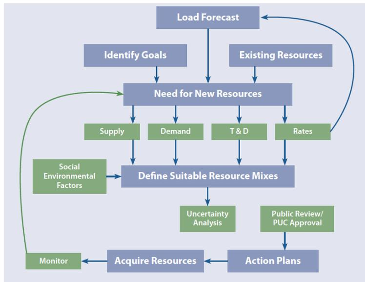
Figure 2-11: Flow Chart for Integrated Resource Planning [7]
