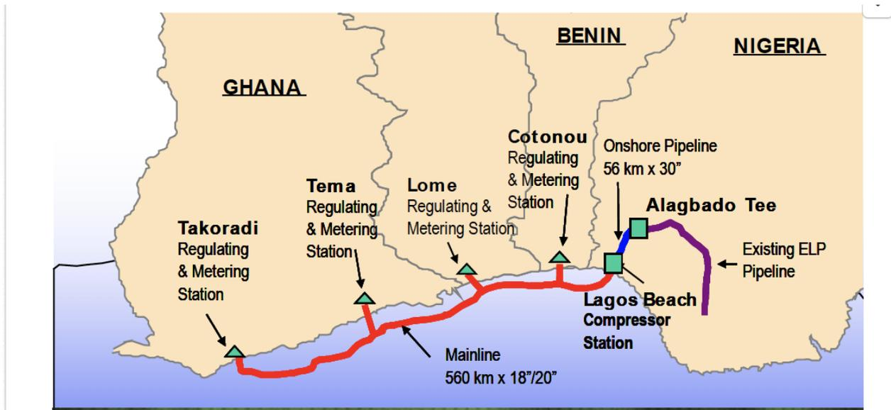
Figure 2-9: West African Gas Pipeline for Gas Supply to Ghana [5]
