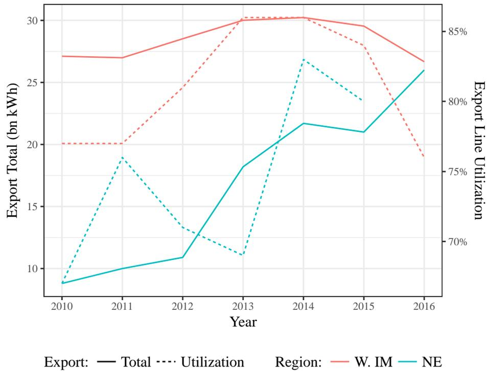
Figure 3.15: Exports to North Grid from W. IM and Northeast Grid. Source: author’s calculation based on NEA, State Grid exchange reports, W. IM Grid reports. Note: the Suizhong coal plant in NE was connected directly to North Grid mid-2015, thus there is no clear line utilization percentage for 2016.
