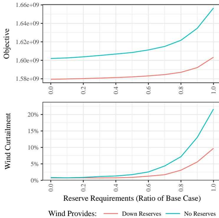
Figure 5.8: Objectives and wind curtailment for range of reserve requirements and wind reserve ability in reference case, Northeast.
