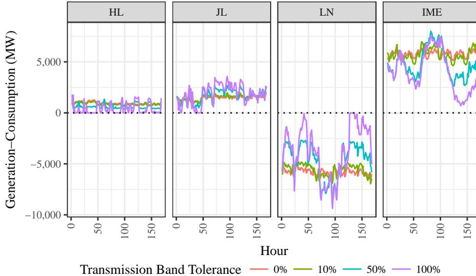
Figure 5.11: Net excess generation by province for transmission band tolerance sensitivity, Northeast PTQ run. (A15Ja1 wind profile)
