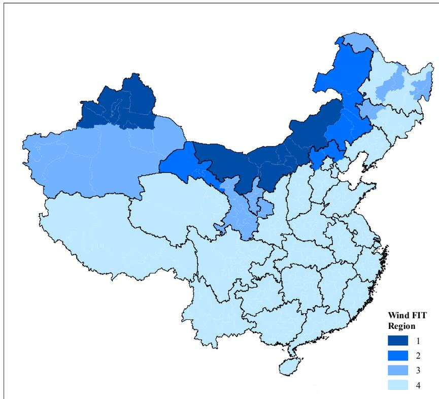
Figure 3.1: Wind feed-in-tariff (FIT) regions of China. New builds in 2017 in tiers 1-4 received 0.47, 0.50, 0.54 and 0.60 yuan / kWh, respectively. Source: (NDRC, 2015c)
