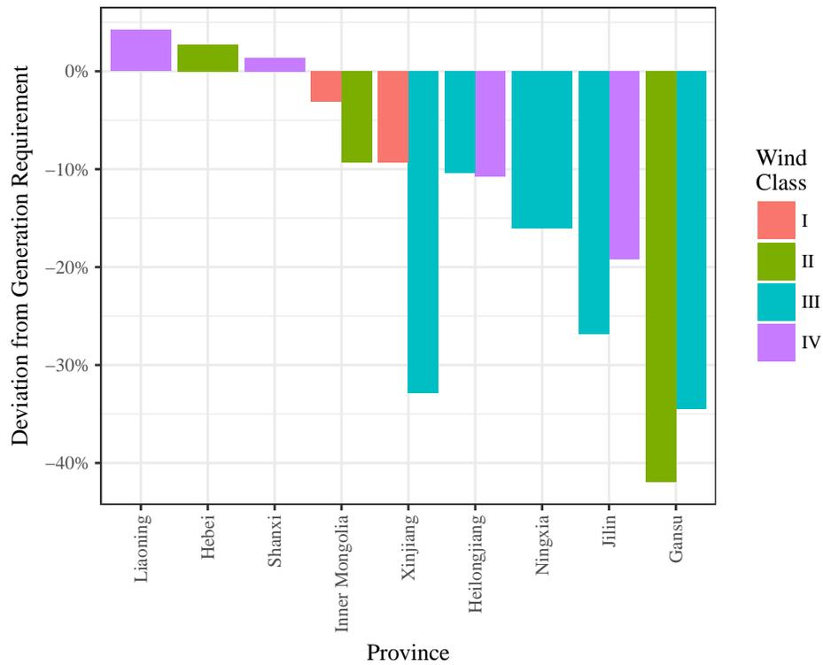
Figure 3.2: Wind generation deviations with respect to minimum capacity factor requirements by province and wind class (I-highest, IV-lowest), 2016. As discussed in the text, these do not consider the tariff paid to wind generators, such as what share is paid through below-benchmark market mechanisms. Source: (NEA, 2017b).
