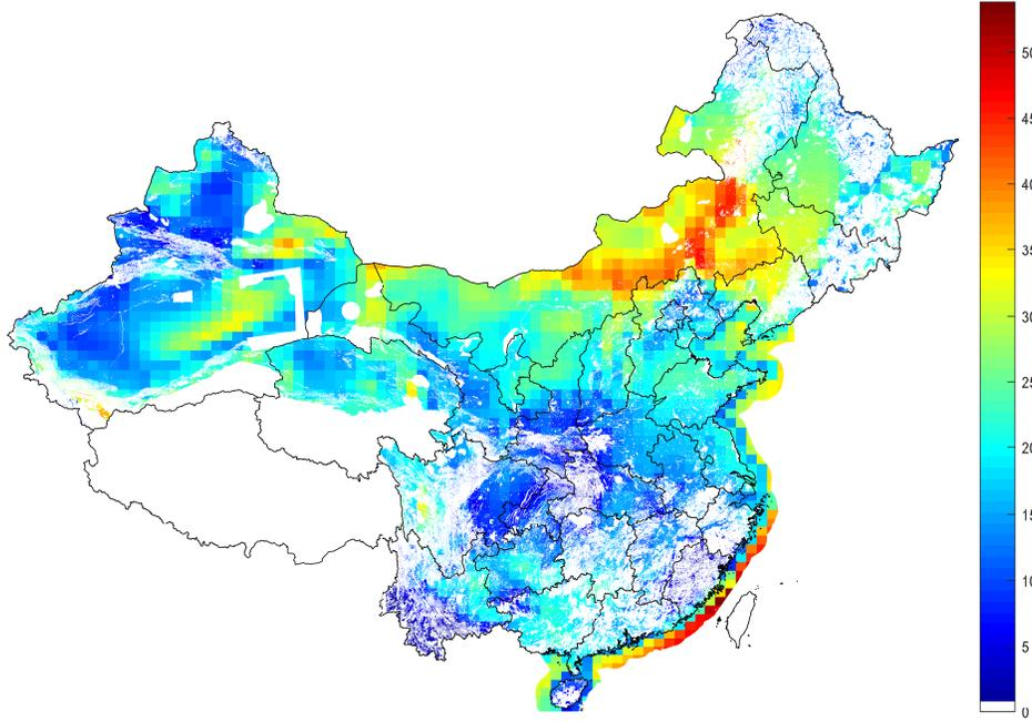
Figure 4.3: Wind capacity factors (%) in China constructed using MERRA, 1979-2015 average. (White areas are deemed unsuitable for wind development.) Source: (Davidson et al., 2016b).
