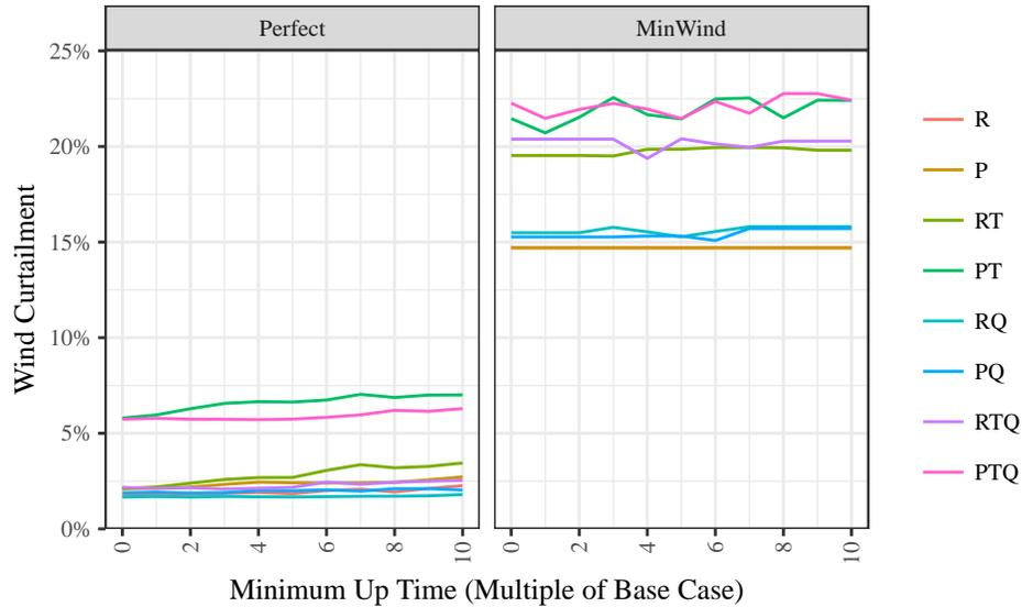
Figure 5.17: Curtailment of minimum up time sensitivity for different scheduling assumptions, Northeast.
