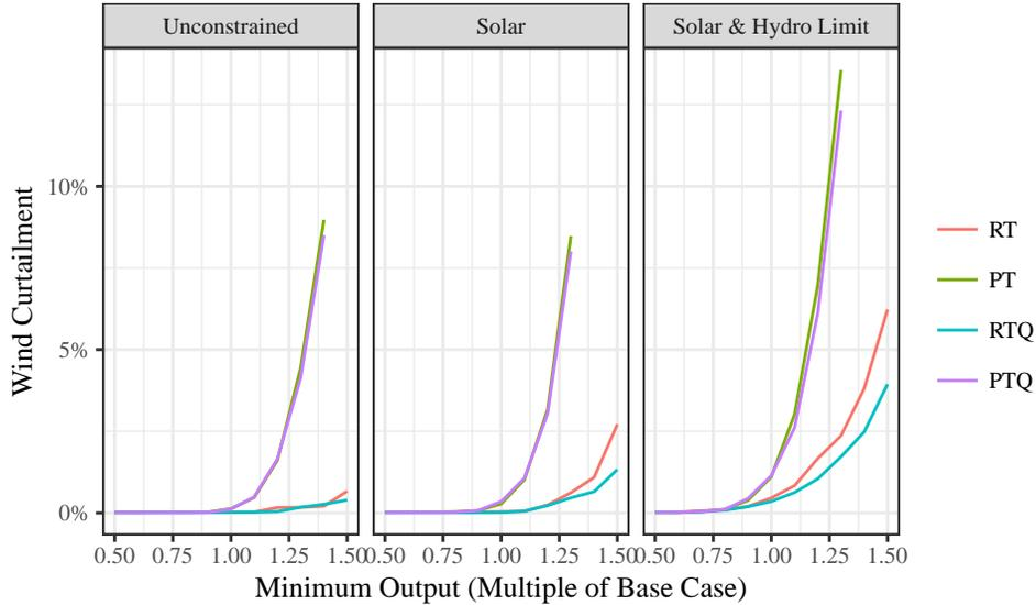
Figure 5.39: Curtailment rates for (conventional unit) minimum output sensitivity with unconstrained (full hydro and no solar), solar, and solar with hydro limits (default), Northwest restricted transmission cases.
