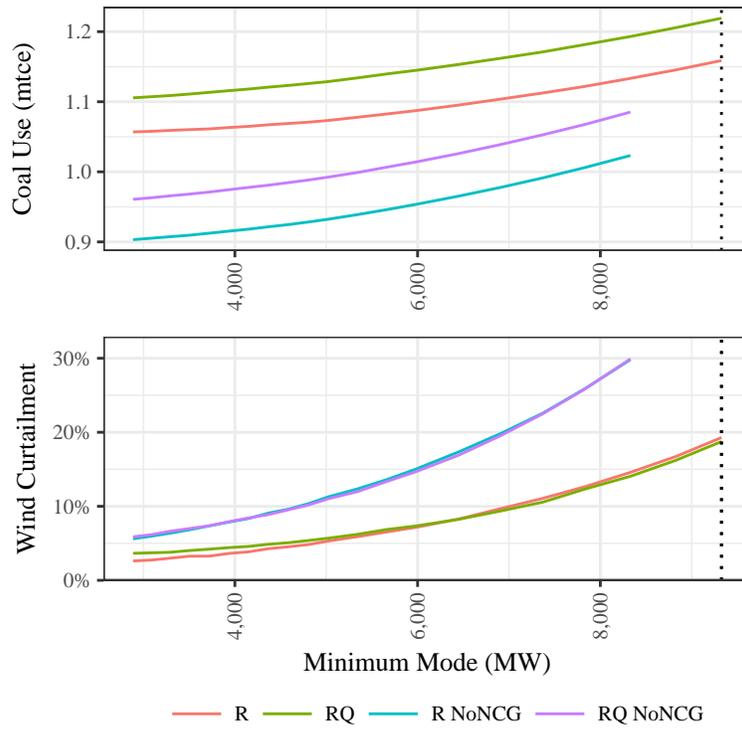
Figure 5.26: Coal use and curtailment with and without North China Grid (NCG) exports for CHP sensitivity, W. Inner Mongolia.
