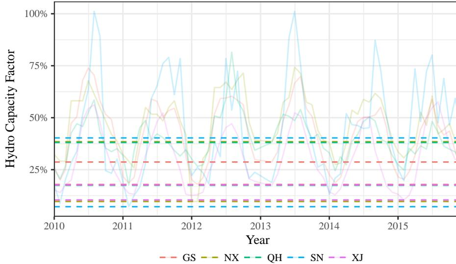
Figure 5.30: Monthly hydro capacity factors and minimum / maximum (dashed) for 2010-2015 winters. Source: (NBS, 2016).
