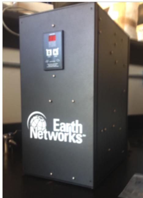
**Figure 2.4:** Earth Networks sampling and drying unit
