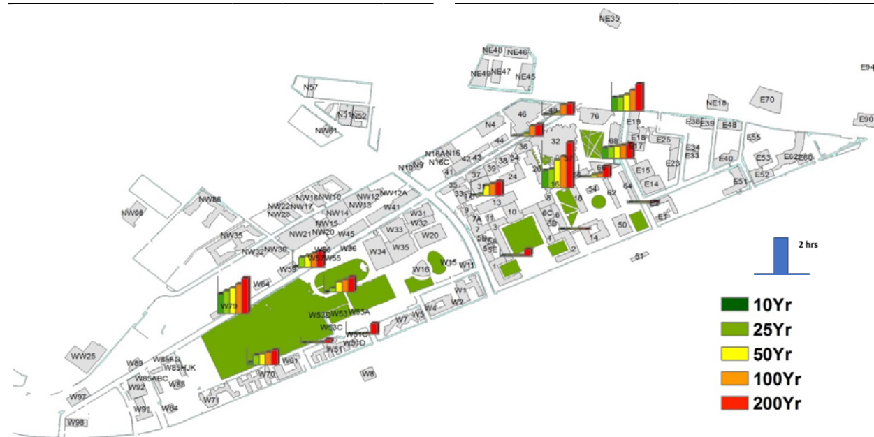
Figure 5. Current flood risk: Hours of Flooding at a sample of manhole locations on campus.
