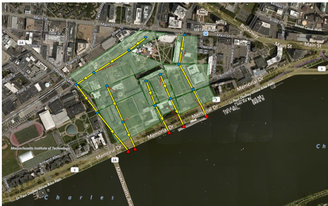
Figure 4. Sample Schematic of MIT Campus Stormwater Infrastructure in PCSWMM
