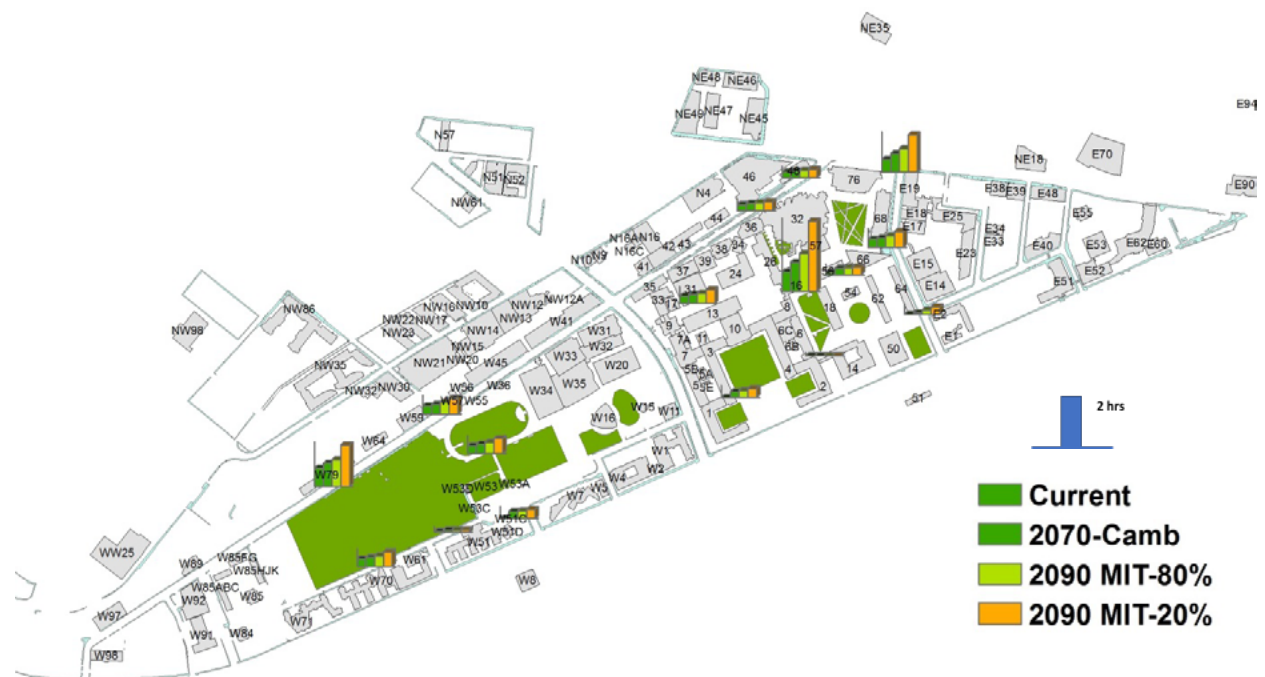
Figure 6. Future projected change in 100-year flood and resulting hours of flooding at key manholes on campus.
