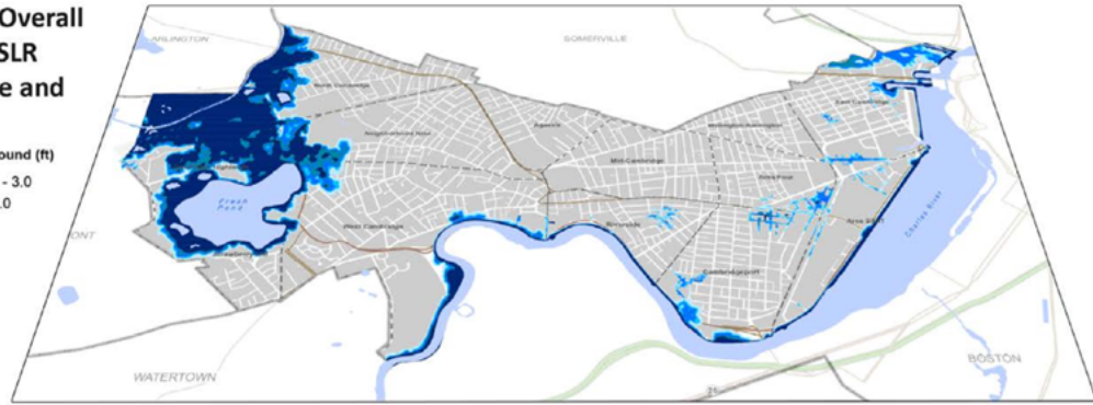
Figure 7. 2070 Depth of Overall flooding from the 100 year SLR/Storm Surge Event (CCVA 2070)
